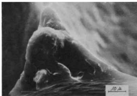
Fig. 3. PUR foam containing 10 wt% of alumina (BACO FRF30) coated with a polyether (1000 MW) unreactive toward isocyanate.
