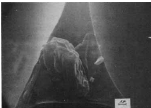
Fig. 2. PUR foam containing 10 wt % of untreated alumina (BACO FRF30).
