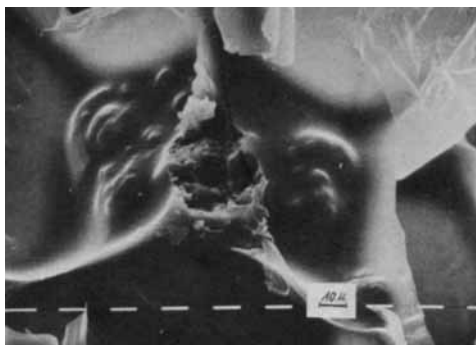
Fig. 4. PUR foam containing 10 wt % of untreated alumina (Merck).
